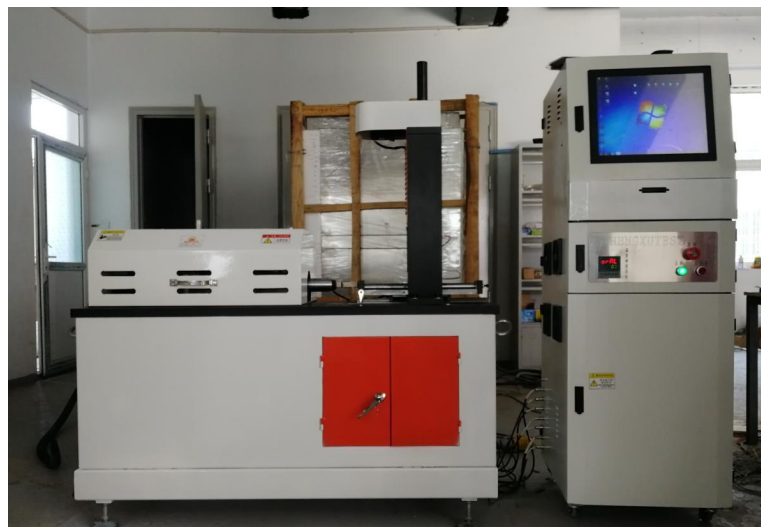
1-Loading unit; 2-Sample and clamping; 3-Measurement of friction force;4-Reciprocating control unit; 5-Host support; 6-Control unit
