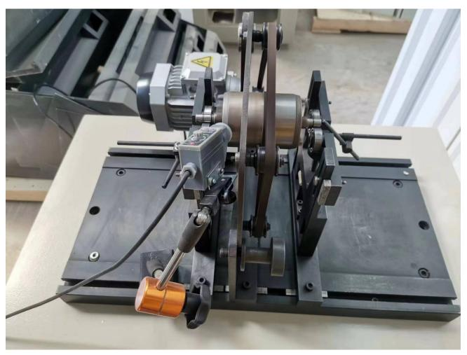
YYQ-5 Horizontal Circle Driven Balance Testing Machine
